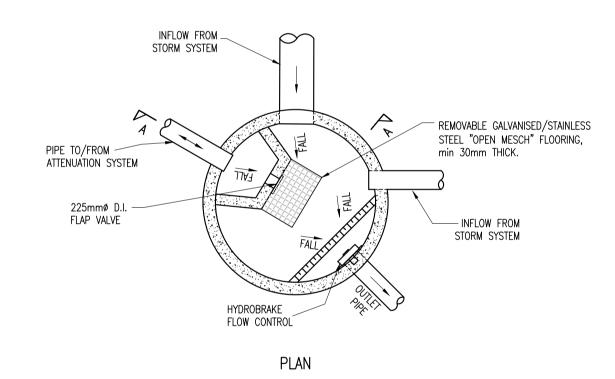
SMART / HYDROBRAKE MANHOLE SCALE 1:50
